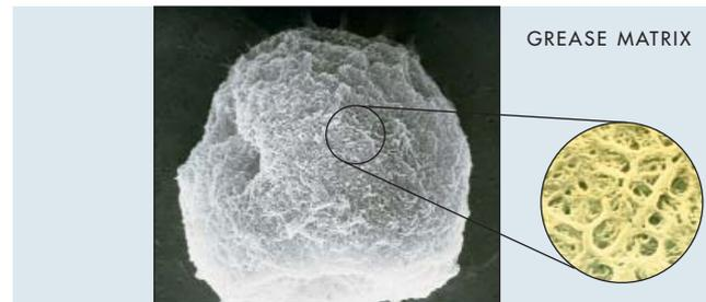
There are three basic components that contribute to the multi-phase structure of lubricating grease; a base fluid, a thickener and very frequently, in modern grease, a group of additives.
