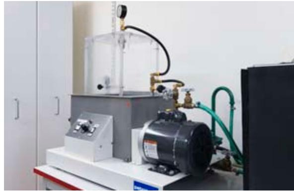
ASTM D 4049, WATER SPRAY OFF TEST APPARATUS
