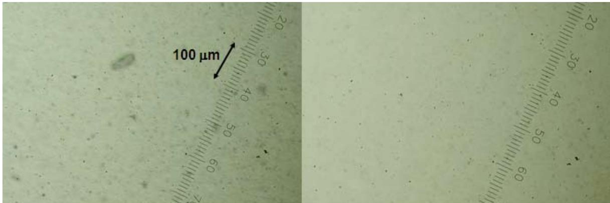
FIGURE 7 – MICROSCOPIC COMPARISON OF TYPICAL AND “CLEAN” GREASES
