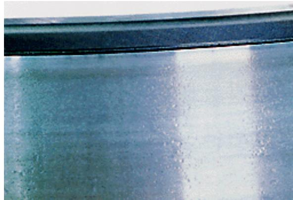
FIGURE 5 – DEBRIS DENTING
