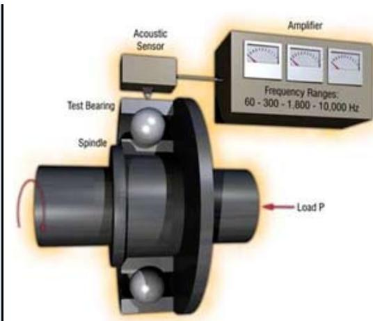
FIGURE 11 – ACOUSTIC GREASE NOISE MEASUREMENT
