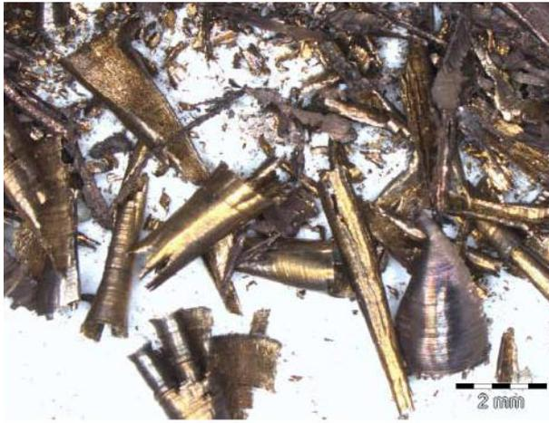
FIGURE 1 – METALLIC MACHINING DEBRIS
