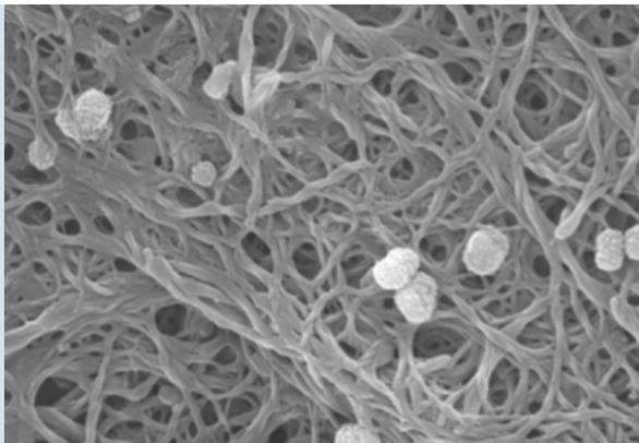
FIGURE 4 – UNREACTED LIME PARTICLES IN SOAP THICKENER MATRIX
