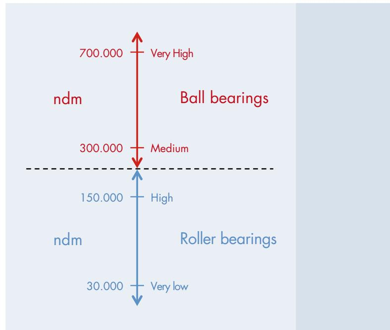
There is unfortunately no standardized way of correlating the speed factor with the structure of the various types of lubricating grease so, for the moment, it can only function as a guideline. The calculation models commonly used only take the base oil viscosity into account and not the thickener type nor the amount. In reality, this will result in a thicker lubricating film than calculated.
