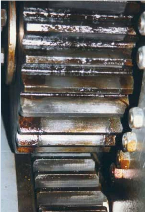
On the other hand, large bearings, typically roller bearings, operate at low speeds and are usually heavily loaded. Support roller bearings in the steel industry are one example of such bearings. For these applications, it is preferable to use a soft product with a high base oil viscosity. It is very likely that the grease needs a high mechanical stability and also a good extreme pressure additive to cope with the high loads.
