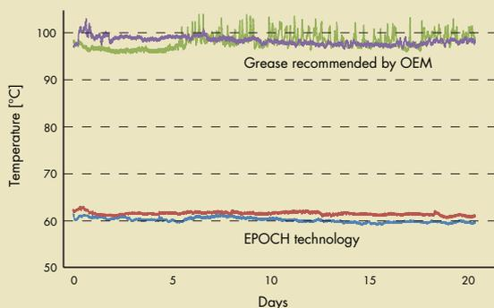
Powertrain has succeeded in reducing the bearing temperature of the flue gas fan by an additional 10 °C, down to an operating temperature of 60°C and this trail will continue until mid-2012.
